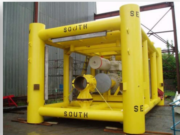
Subsea isolation valve structure
