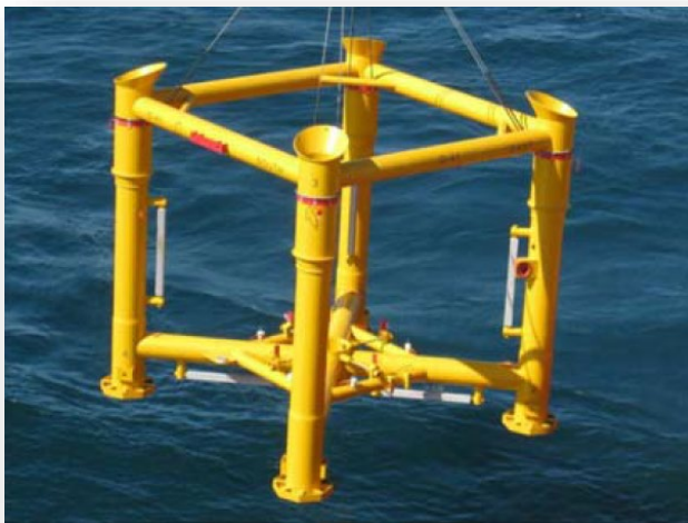
Wellhead protection structure
