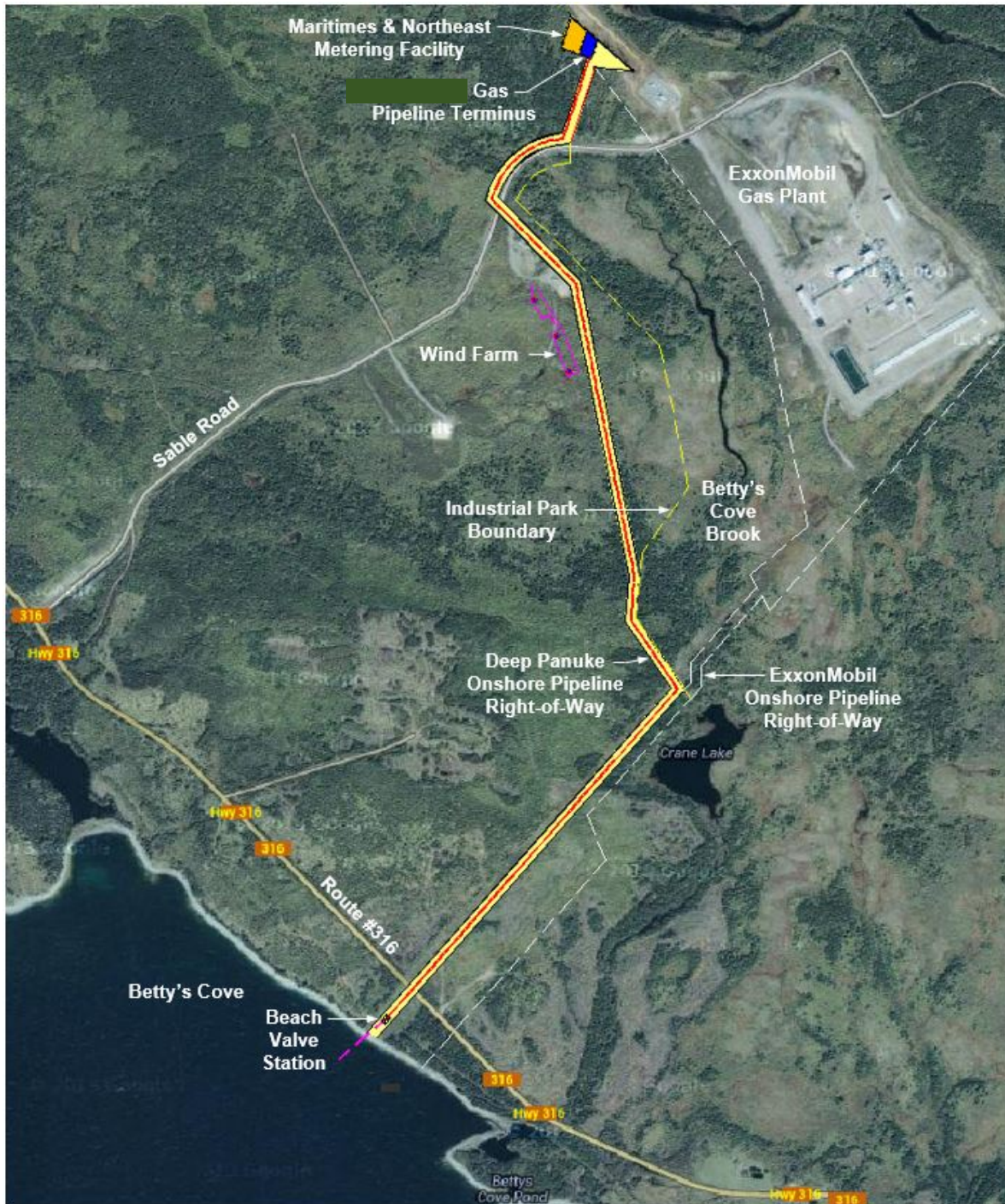
Onshore Portion of the Deep Panuke Gas Pipeline
