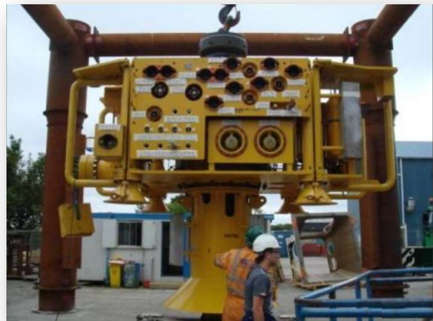
Typical Subsea Tree
