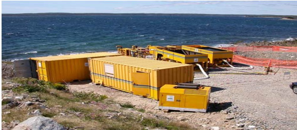
Example of the type of pumping equipment that will be used at landfall during the GEP flushing program
