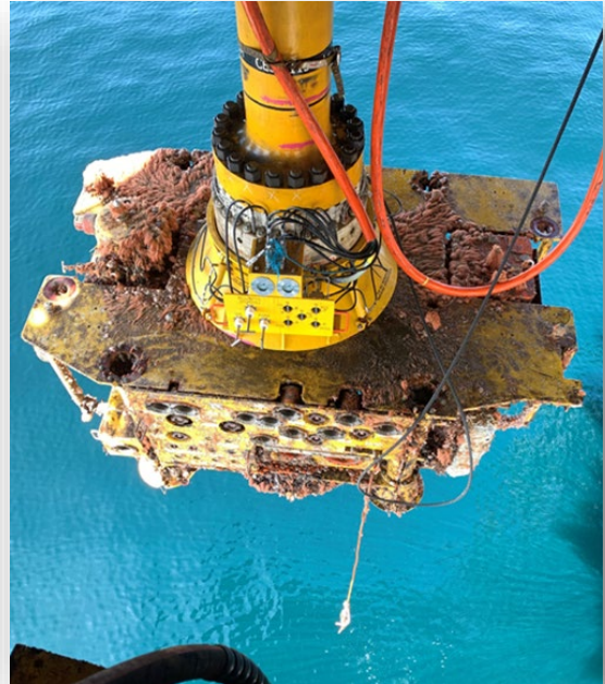
Recovered Well Subsea Tree
